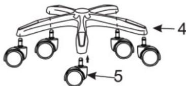
**2. Place the gas lift into the star base. Place the gas lift cover over the gas lift.**
