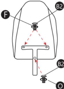
**7. Insert the backrest mount into the hole in the butterfly mechanism and secure it by turning the handle**
