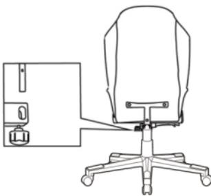
**8. Fasten the armrests with screws C. Close the screw holes with caps E.**
