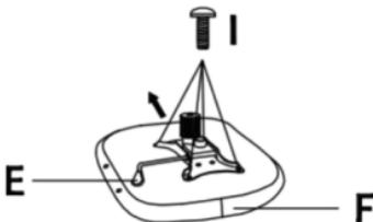
**3. Place the seat on the gas lift C**
