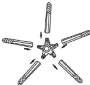
**2. Push and twist the casters into the star base. Place the gas lift into the star base. Place the gas lift cover over the gas lift.**
