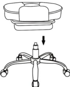
**6. Insert the backrest mount into the hole in the butterfly mechanism and secure it by turning the handle.**
