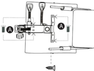
**5. Fasten the backrest mount 8 to the back of the backrest 1 with screws G and shims C.**
