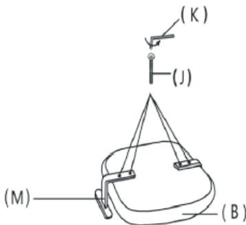
**3. Fasten the backrest A to the seat B mountings. Do this on both sides of the backrest A. Use the screws J and hex wrench K.**
