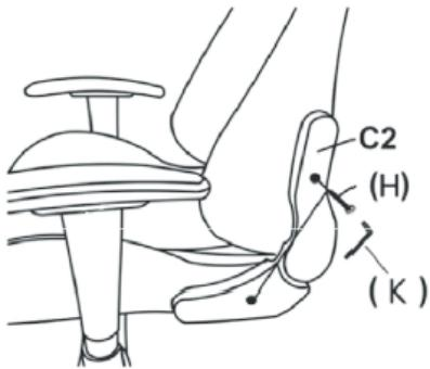
**5. Fasten the butterfly mechanism over the seat B. Use the screws J and hex wrench K.**
